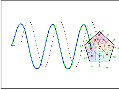
Fig. 3. Simulation results by implementing Lloyd’s algorithm (5) and leader-follower consensus protocol (20). A polygon domain is moving along a sinusoidal trajectory, i.e., the black dashed line “- -”; the trajectory of a randomly selected agent (denoted as red “★”) is denoted by the blue solid line “—” and green dashed line “- -” when implementing Lloyd’s algorithm and leader-follower consensus protocol respectively.
